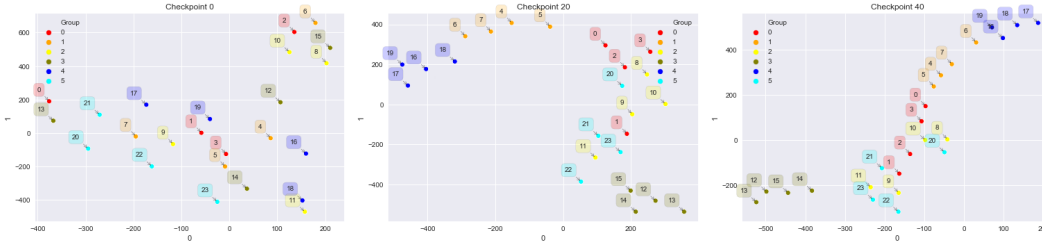
Figure 4: Policy divergence over time. T-SNE visualization of policy divergences over 40 training updates. Colors denote original latent group. Computing pairwise distances using our divergence metric leads to noticeable grouping over time.
