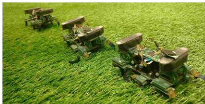
Figure 1: We implement our sample-efficient meta-reinforcement learning algorithm on a real legged millirobot, enabling online adaptation to new tasks and unexpected occurrences such as losing a leg.
